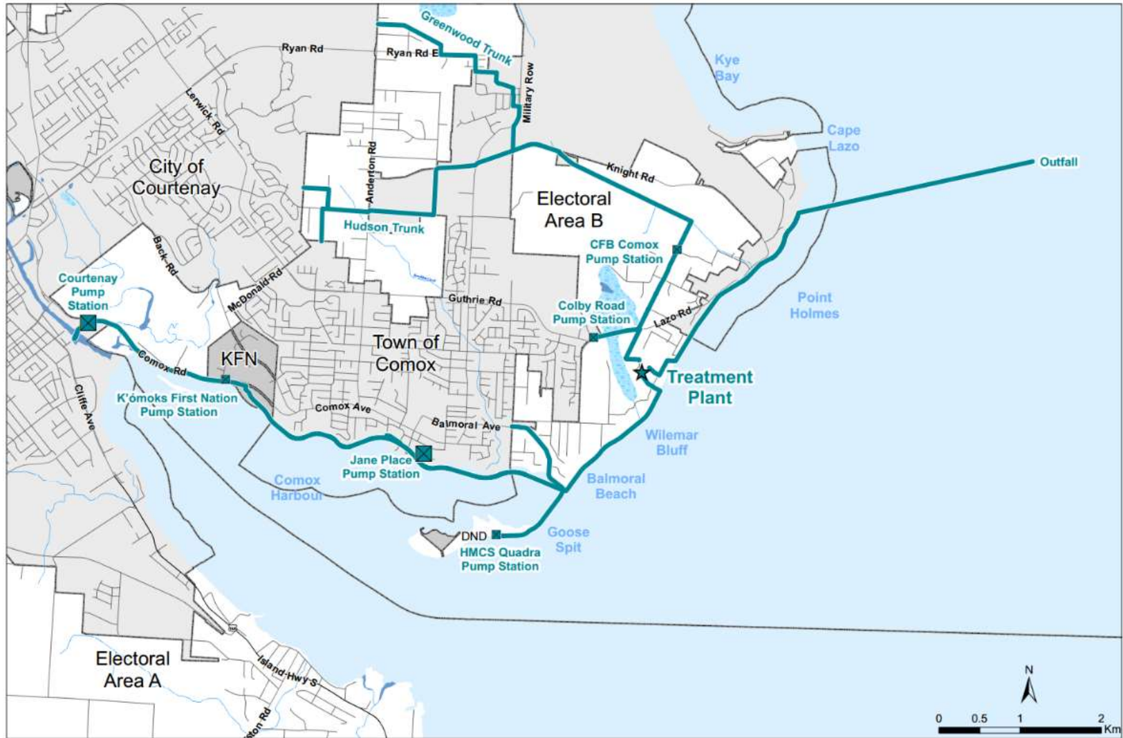
Figure 10-1: Existing Force Main Alignment
